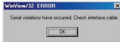
Figure 67. Serial Violations Have Occurred dialog box
