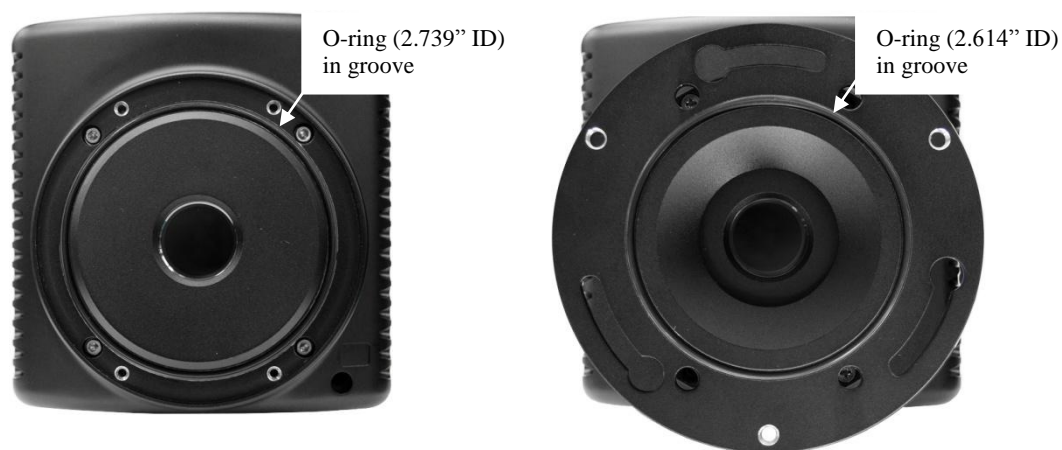
Figure 124. O-ring Positions for PI-MAX3 NVUV Cameras
